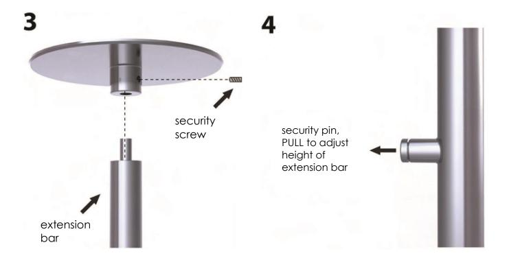
3 - Screw in extension bar system into base and secure it with the side security screw.
