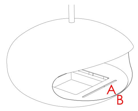
NOTE: adjustment instructions on the following page showing relative positions of (A) and (B) shown above are critical to the airflow inside the *Main Body* and therefore critical to the proper functioning of the *Combustion Chamber*.
