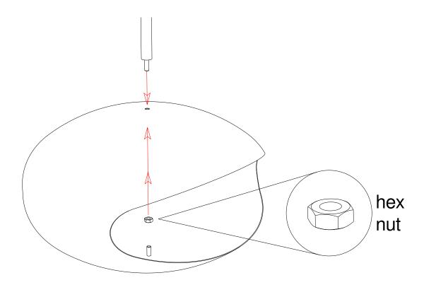
Position Main Body into hanging bar and secure from inside with hex type nut.
