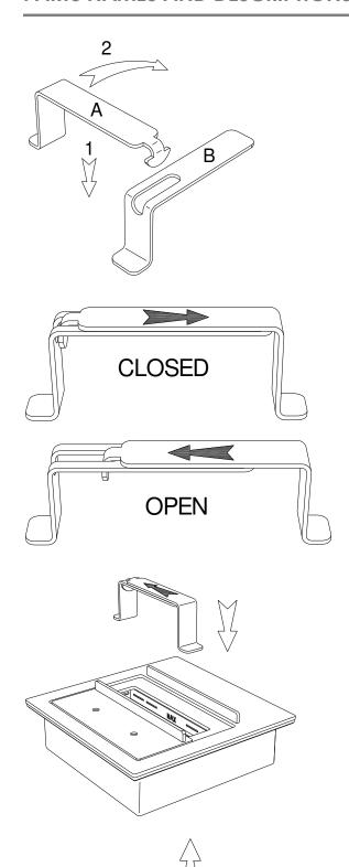
The Lifting Handle is used to take the Combustion Chamber in and out of the Mount Plate inside the Main Body for filling and cleaning. Step 1 is to join Part A and Part B as shown to the left. Once you have placed the tag of Part A into the slot of Part B, then twist it 90 degrees to lock them as one handle.
