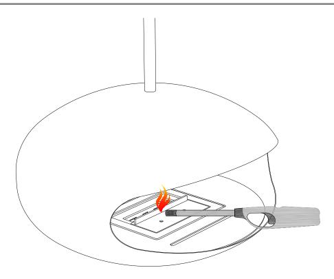
Using a long arm fire lighter and standing at a safe distance from the Combustion Chamber carefully introduce a flame as indicated above to ignite the Combustion Chamber. Always make sure there is a Class B fire extinguisher close at hand when igniting the Combustion Chamber.
