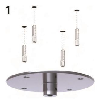
1 - Mark and drill 4 holes in the ceiling and insert the corresponding dowels into the holes (Dowels are not provided).
